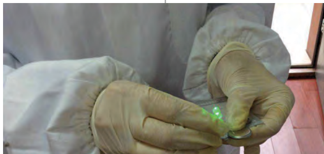
Demonstration of LED energized by one of the first solid polymer HNT lithium batteries being developed at the College of Mines and Earth Sciences at the University of Utah.
